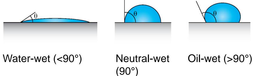
In an oil reservoir, the surfaces of the grains which make the matrix of the reservoir may be oil-, water- or mixed-wet, illustrated below.
